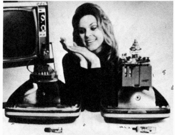
Fig. 14: Comparison of the new tube with its integral deflection yoke on the left and on the right a conventional delta gun shadowmask tube. Note that it is common US practice to mount the convergence controls on the deflection/convergence assembly with standard delta gun shadowmask tubes.
