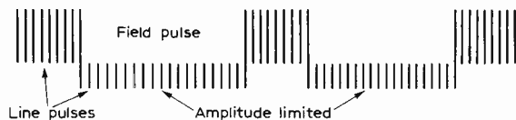
Fig. 6: Non-interlaced field sync pulse.
