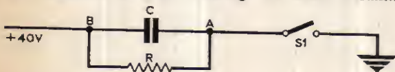
Fig. 6: Equivalent circuit of a portion of the vidicon target. The action of the electron beam is to close S1 momentarily so that side A of capacitor C is earthed. Current flowing through resistor R restores A to +40V but not before S1 has been closed again by the beam. The voltage reached at A depends on the value of R and so on the light received. Whenever S1 is closed and A discharges to earth, a current flows to plate B. This current is the output of the vidicon.
