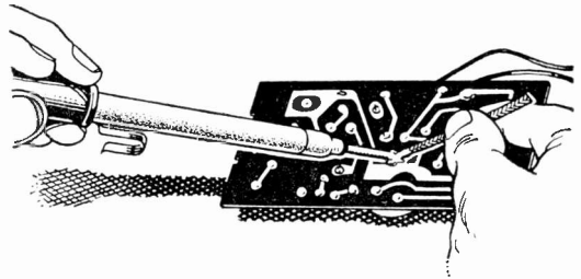
Using copper braiding to absorb solder
