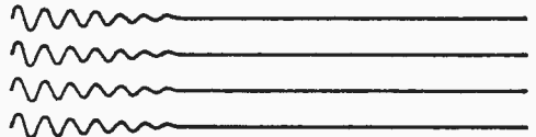
Fig. 4—The effect on the horizontal pictures lines caused by velocity modulation of the frame scanning current waveform.
