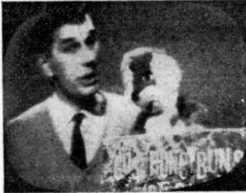
Fig. 3—This picture shows a television picture with a signal/noise ratio of about 30 to 1.
