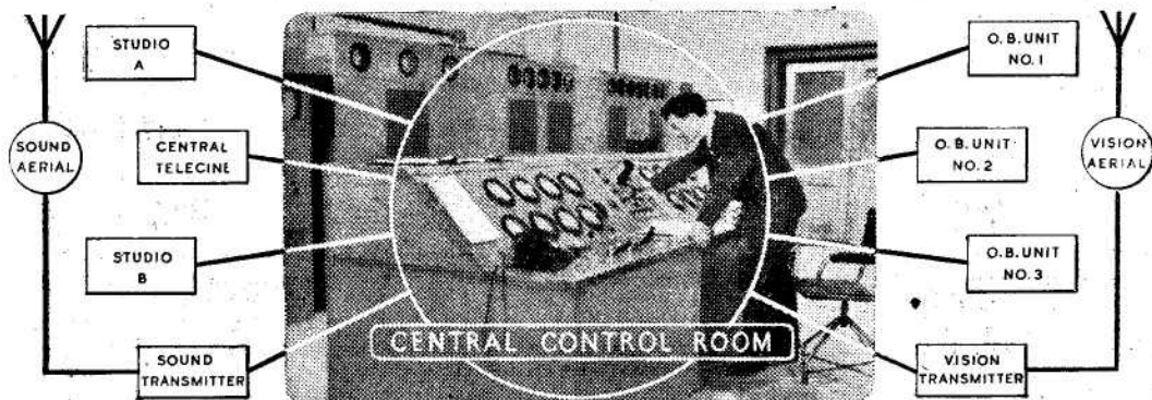
The control room and its links shown diagrammatically.
