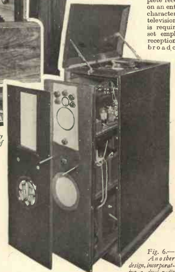
Fig. 6.—Another design, incorporating a dual radio receiver with a cathode-ray tube for building up the television images.
