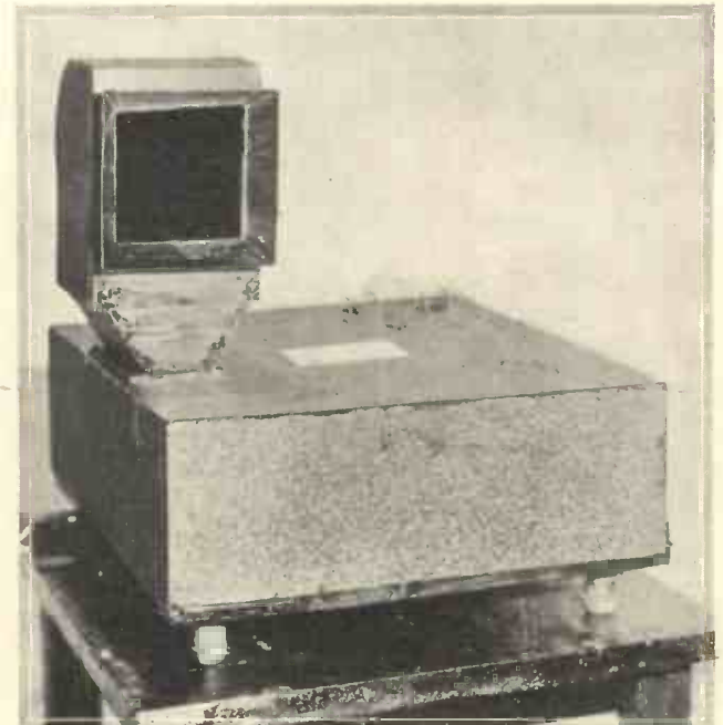
Fig. 1.—By mounting the motor vertically and the disc and neon lamp horizontally, the image can be observed at the top of the cowl via a periscopic mirror
