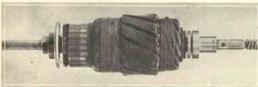
Fig. 4.—"Skewing" or inclining the armature slots of a television motor is sound practice.
