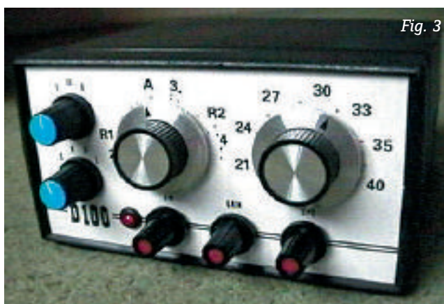
A D-100 DX-TV converter inverts French video before it enters the TV receiver
