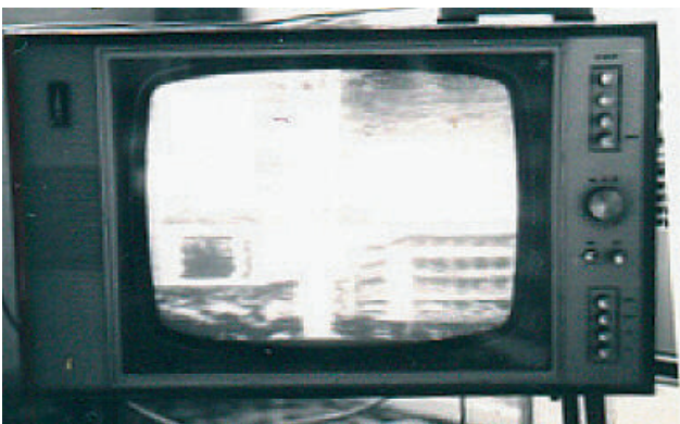
A Bush TV125 dual-standard receiver displaying a Yugoslavian identification caption (TV Beograd) circa 1972
