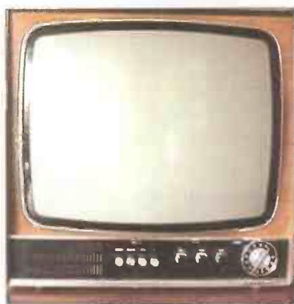
Above: The Ferguson 3660, one of the last dual-standard TV receivers to be manufactured, fitted with the Thorn (BRC) 1400 Series chassis.
