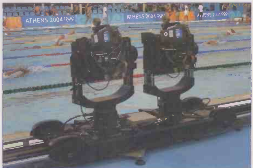
Camera Tracking Company's G2W rail system, unveiled at the Athens Olympics 2004, is specifically designed for coverage of Swimming.
