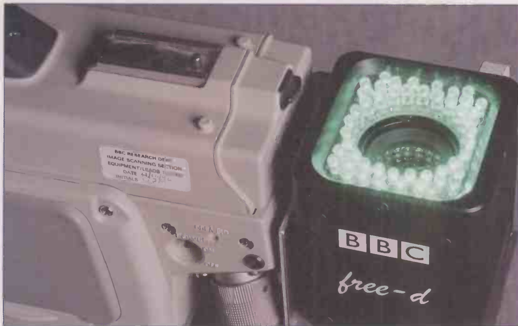
Figure 2. The markers are viewed by a small auxiliary camera mounted on the side of each normal studio camera.
