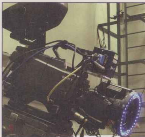
Figure 5. To change the key colour, it is only necessary to change the lights on the cameras; there is no need to change the whole cyclorama.
