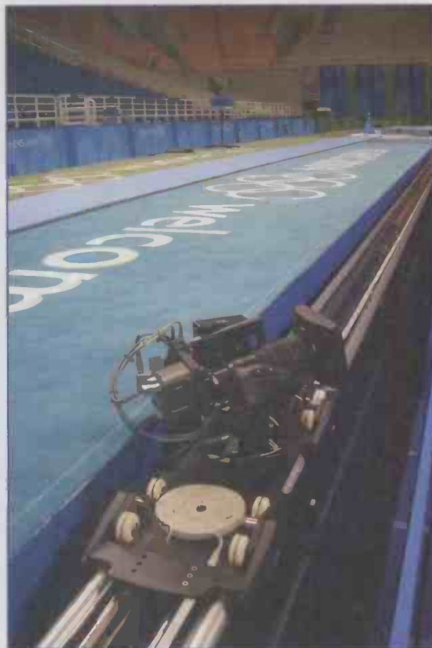
The MG2 rail system is a compact and lightweight tracking system which can currently run over lengths of up to 30m.
