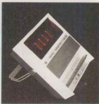
the DA114 used neon-filled Nixie numerical display tubes
