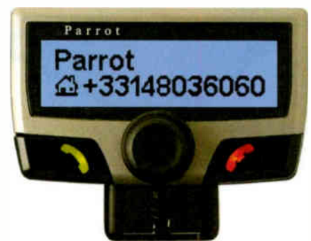
Photo 4: The Parrot CK3100 hands-free in-car kit provides visual information as well as routine mobile-phone functions.
