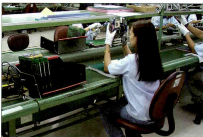
Quality-control inspection of lead-free soldered PCBs. Note the rework equipment at the left.
