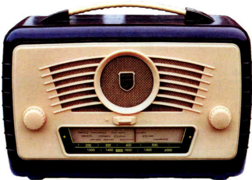
Appearance of the Ultra Coronation Twin receiver after attention to the cabinet and tuning scale.
