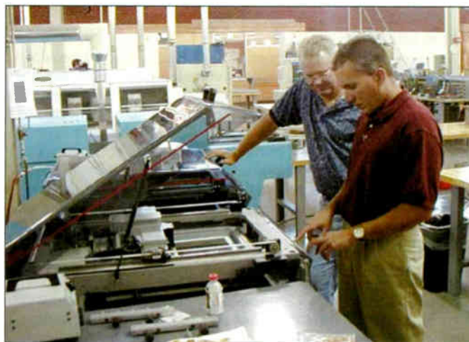
A wave-soldering station that uses lead-free solder.
