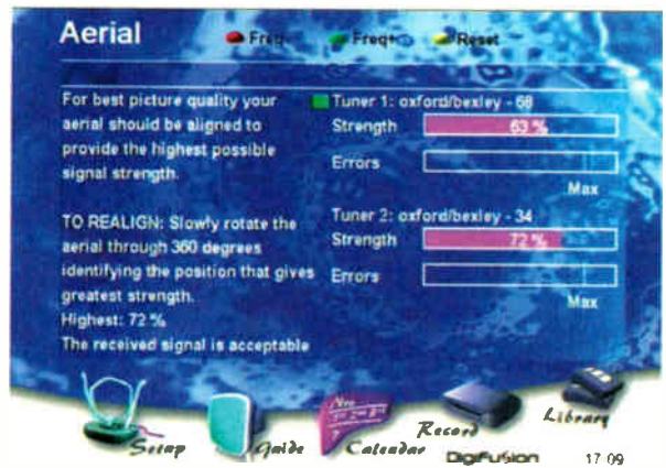
Photo 2: The aerial-alignment option that can be selected from the setup menu.
