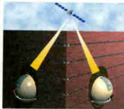
Figure 6: Reception from three satellites with the JSAT hemispherical Luneberg-lens aerial.
