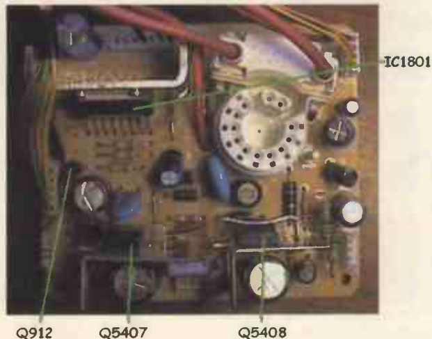
Fig. 19: Position of CRT base PCB components that can fail under high-HT conditions.
