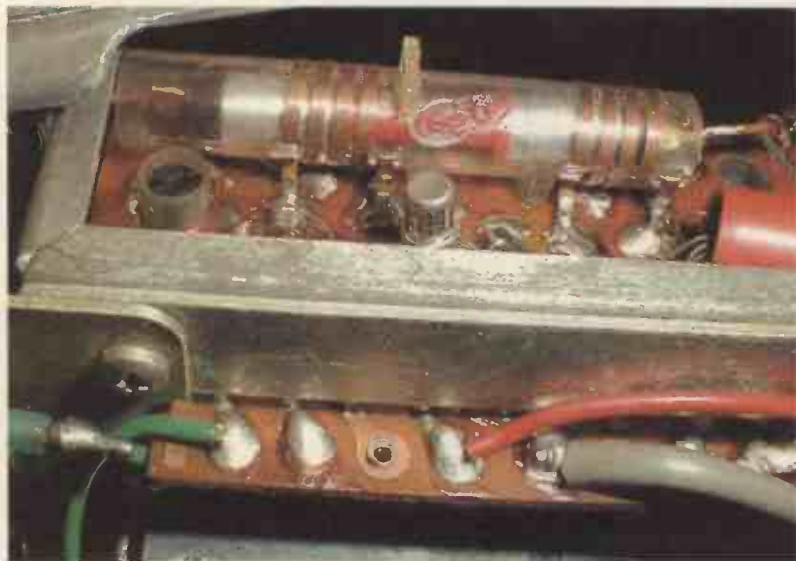
Photo 3: The VHF tuner, after removal of its screening can.
