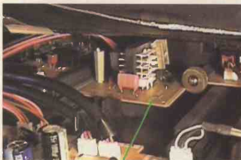
Fig. 15: Location of the power-factor correction PCB in Model 56FW53H.
