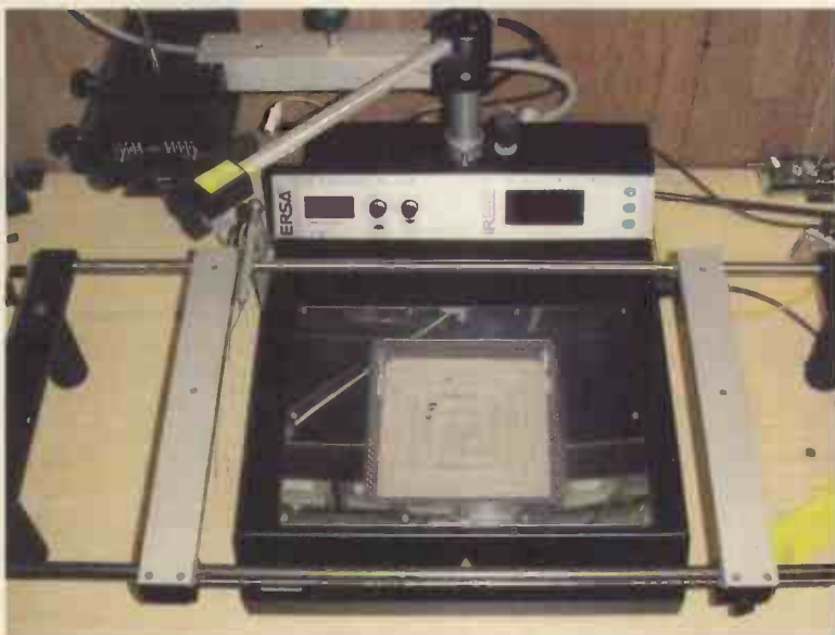
Photo 1: Michael Dranfield's ERSA IR500A PCB rework station. The overhead radiator is at top left.
