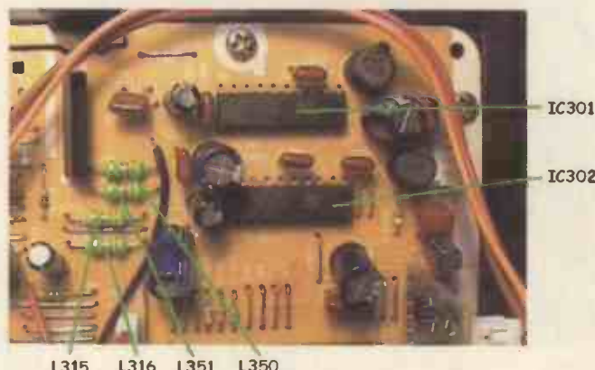
Fig. 17: Location of the audio output stage components on the main PCB.
