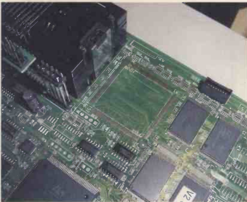
Photo 4: PCB after removal of a 208-pin IC and cleaning up with desoldering braid. No PCB or track damage has occurred.
