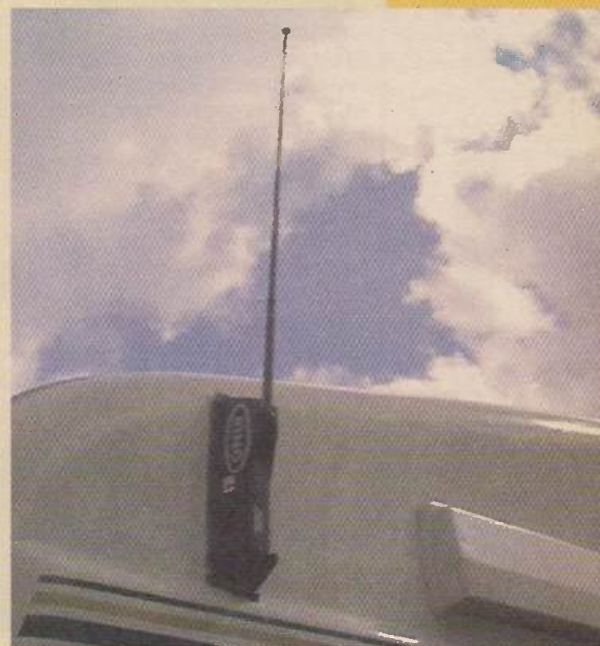
An amplified electrical aerial mounted on the outside of a caravan.
