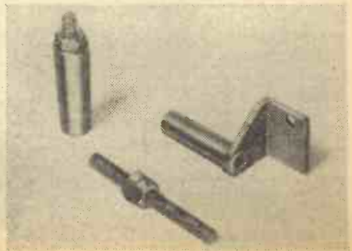
Mandrel socket stop with adjustable saddle stop and bracket.
