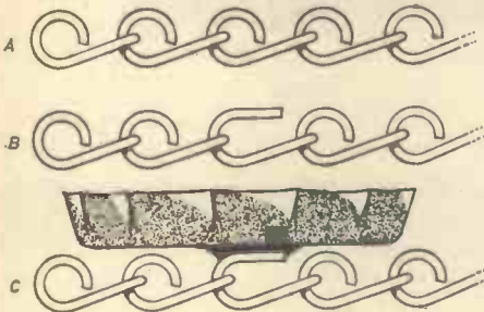
Fig. 3. In B an end link of the chain A is shown opened for attachment to the end of another length of chain. C, side view of bottle cap soldered to a link of the chain for use as food container.
