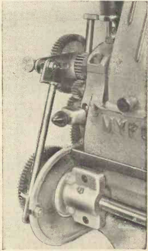
Operator's view of dividing attachment set up.
