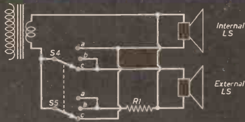
Fig. 163.—Circuit to allow use of either speaker or both with the volume remaining constant.
