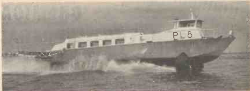
Fig. 8.—Hydrofoil craft PL8, capable of carrying 50 passengers at a speed of 35 knots was built for the Shell Petroleum Company in Holland. It operates on Lake Maracaibo, Venezuela. (Photo by courtesy of F. H. van Dijk, Rotterdam.)
