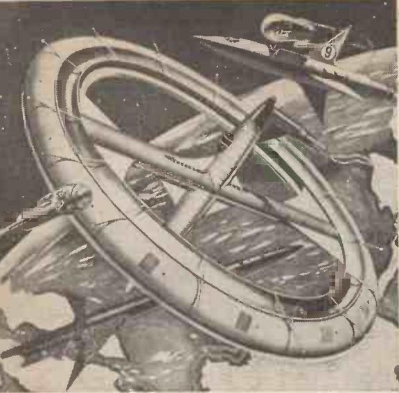
An artist's impression of the space station of the future. It is made of inflated plastic sections and rotates to induce artificial gravity.
