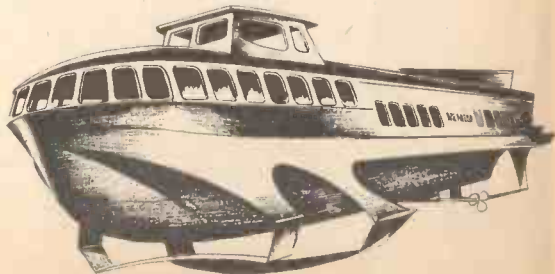
Fig. 2.—The Russian "Meteor" hydrofoil boat can carry 150 passengers at 29 knots.
