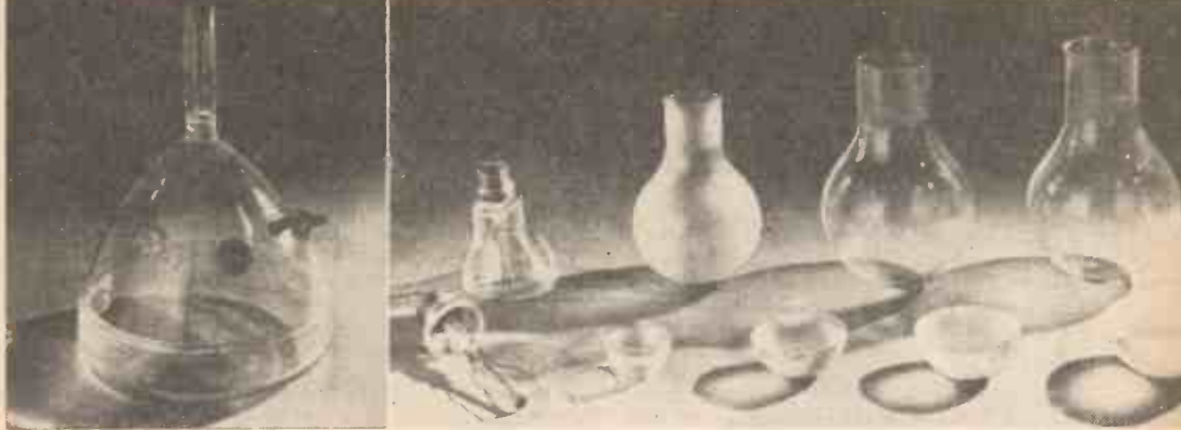
Fig. 39.—Examples of flasks and evaporating dishes made from a television tube and electric light bulbs.
