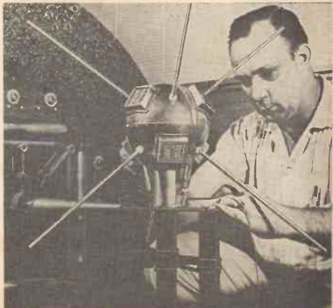
Fig. 6.—Vanguard 1—the first satellite to use solar batteries. Its solar cells are housed in six rectangular "windows."
