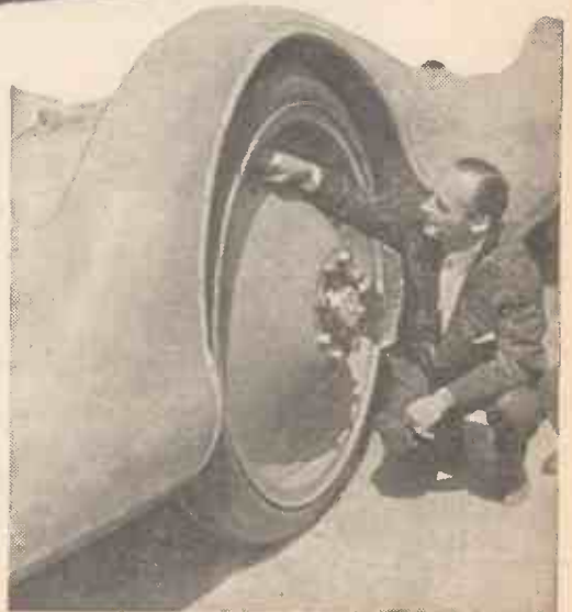
Fig. 5.—Donald Campbell looking at one of the giant 4ft. 4in. dia. front wheels of the "Bluebird."
