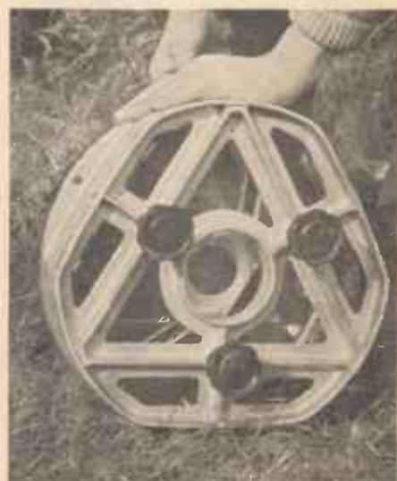
Fig. 8.—Rear view of the primary mirror cell, showing the mirror adjusting screws.
