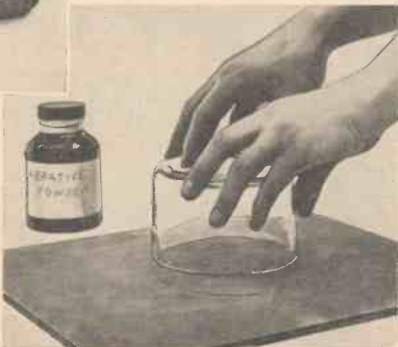
Fig. 9.—Grinding the cut surface smooth using carborundum powder and water on a piece of plate glass.
