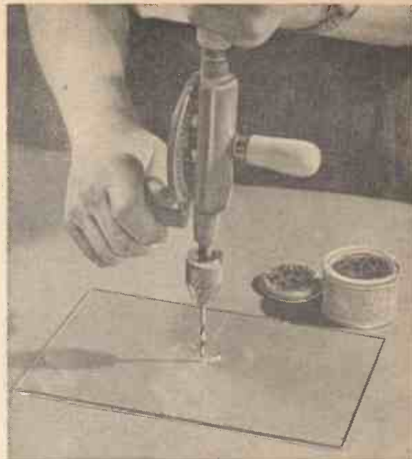
Fig. 7.—A combined abrasive and cooling agent being used whilst drilling plate glass.
