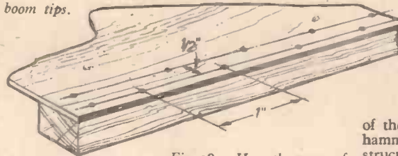
Fig. 18.—How the rows of gimp pins on spar flanges, etc., are staggered.
