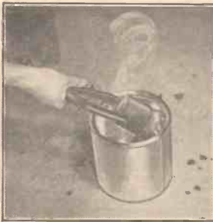
Fig. 10.—The mould is dropped into a can of water.
