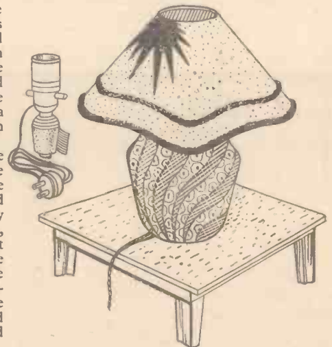
Fig. 5.—Hand-painted ginger jar fitted with a flared hand-painted shade of sheepskin parchment on a wire frame. Also shown is the Pifco adaptor with tapered cork stopper.
