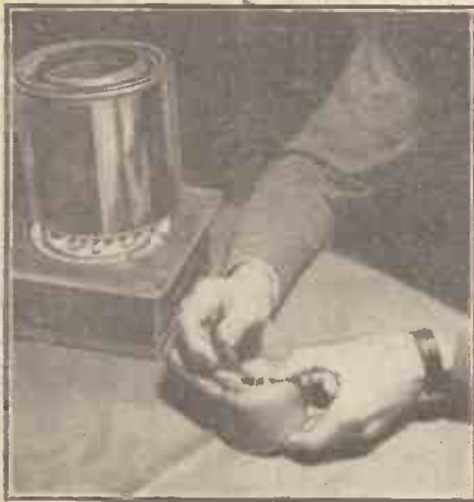
Fig. 1.—Removing the original from the flexible mould. The jacketed container for melting Vinamold can be seen in the background.
