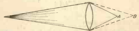
Fig. 9.—Chromatic aberration. A—point of focus of blue rays. B—point of focus of yellow rays.
