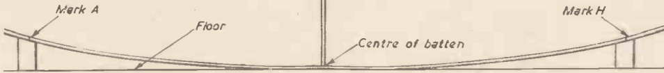
Fig. 19.—The fore and aft curve or sheer of the bottom of the boat.
