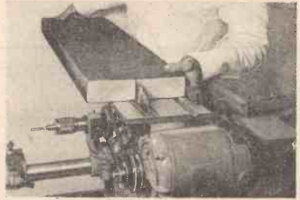
Fig. 4.—The Coronet "Minorette" which used a 1/2 h.p. double-ended motor.
