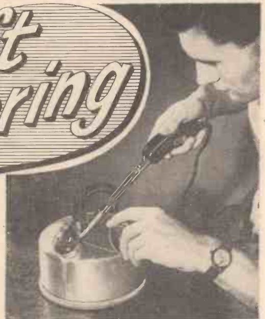
Fig. 2.—Using the point of the bit to direct solder into an angled joint.
