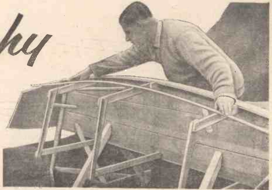
Fig. 10.—Testing the fairing of the frames. This operation will be described next month.
