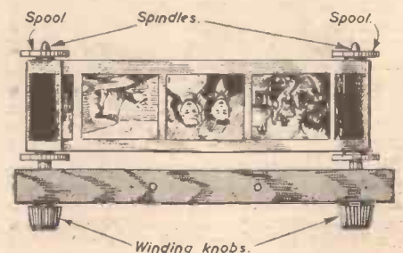
Fig. 4.—Holder for uncut film.
