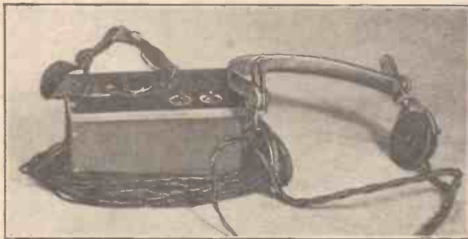
Fig. 2.—The throat microphone, the cased two-valve amplifier and batteries, 60ft. of bell flex and the high impedance earphones.
