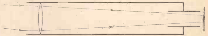
Fig. 1.—The normally accepted way of photographing the moon by placing a photographic plate at the focus of the objective or mirror of a telescope.
