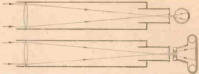
Fig. 4.—The method of photographing the moon recommended in this article. The telescope is focused with the eye and then a miniature camera is substituted.
