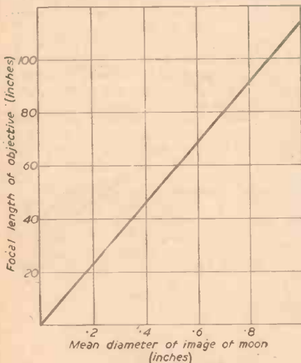
Fig. 2.—Guide to rough diameter of moon image for a given focal length.
