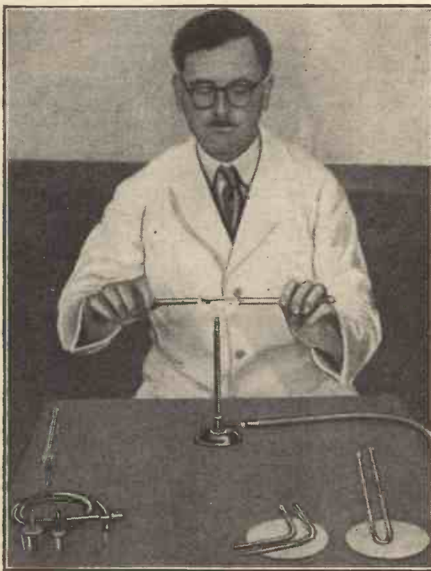
Heating a piece of glass tubing prior to bending. (Note blow-tube and assortment of rubber stoppers in left foreground.)
