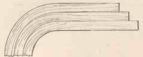
Fig. 6.—Reduction in length of laminae caused by bending.
