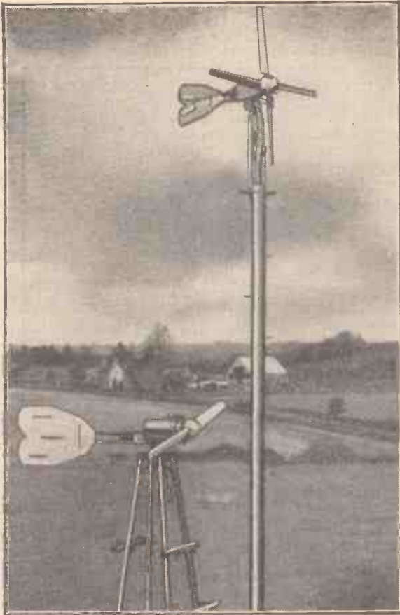
The finished wind-charger unit mounted on a 34 ft. mast. On the left is a two-bladed propeller unit.
