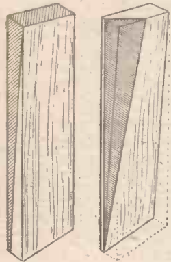
Figs. 5 and 6.—Details of the wooden former for shaping the metal propeller shell.
