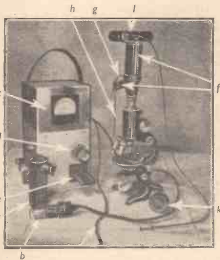
Fig. 2.—Microscope fitted with photomicrographic extension tube and Leica camera. Photomultiplier cell removed from housing.
