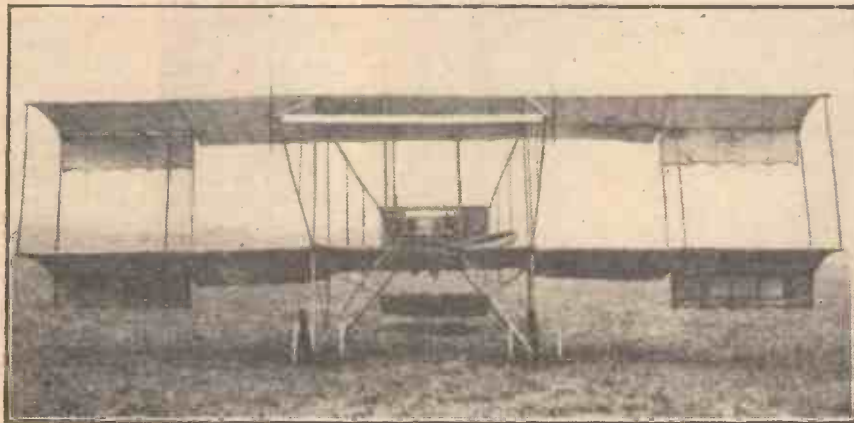
A Grahame-White biplane, commonly known as a "box-kite," built at Hendon, and largely used for elementary training.
