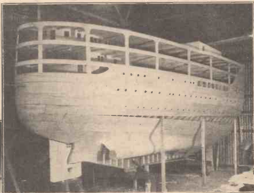
Fig. 2.—This photograph shows the model of the stern portion of the new Orient liner, "Orcades," during plating process on the hull. Scale, 1½ in. to 1ft. (one eighth actual size).
