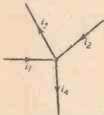
Fig. 1.—Why must the "algebraic sum of currents meeting at a junction" P, always be zero?
