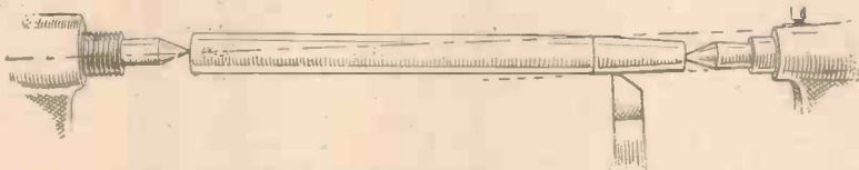
Fig. 40.—Method of setting tail stock for taper turning.
