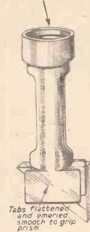
Fig. 11.—Detail of the prism mounting.
