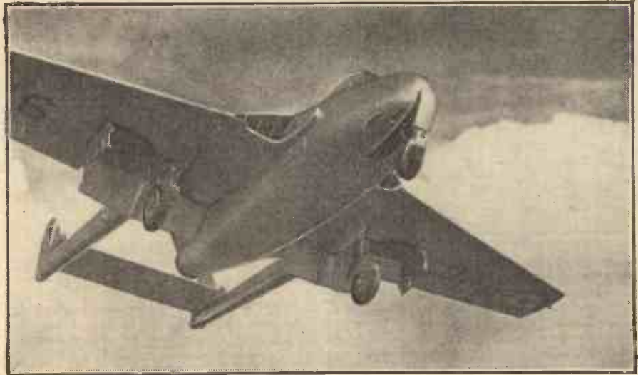
The de Havilland 112 in flight. This aircraft, named the Venom, and powered with a de Havilland ghost jet engine, is a single-seat fighter, and can be used as a fighter-bomber.
