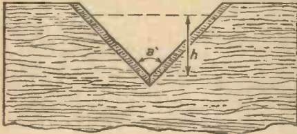
Fig. 1.—Simple measuring weir with triangular notch.
