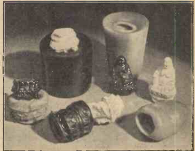
A group of moulds and casts; moulds in background were formed by pouring; moulds in foreground were formed by dipping. Two of the moulds are peeled back to demonstrate elasticity. Dark castings are cold-set resins; light castings are plaster. (Photo: Vinyl Products, Ltd.)
