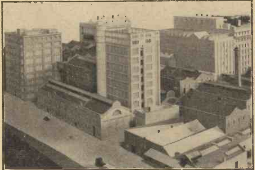
Fig. 3.—A complete view of the fully-detailed architectural model of the factory and warehouses of Messrs. J. Bibby & Sons, Ltd., Liverpool. The model is to a scale of 1/16 in. to 1 ft.
