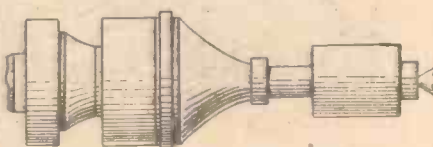
Fig. 78.—Cutting the finial down to lengths and diameters.
