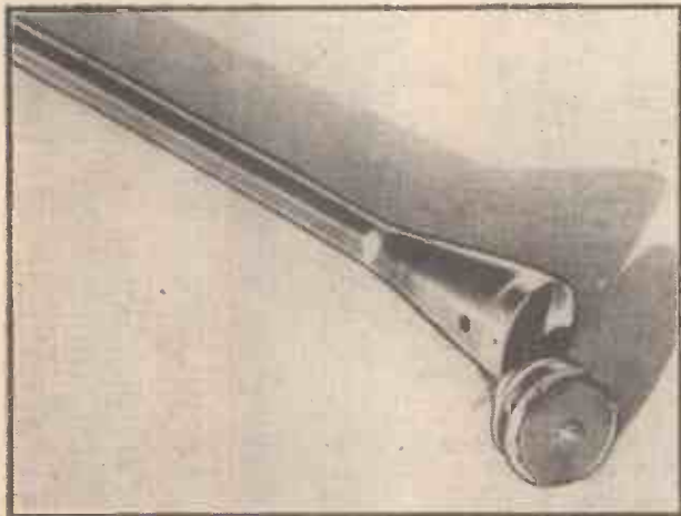
Fig. 30.—The Decojet is noted for its exceptionally easy starting. This is assisted by the long tail pipe. A special feature is the detachable shroud to protect the "flutter-valve" when the engine is being run on a slow model or for long periods at rest. This disc can be seen in the photograph attached to the head, which is shown detached in front of its combustion chamber.
