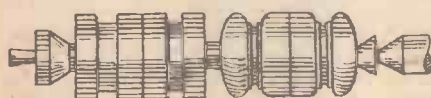
Fig. 62.—Two mallet heads may be turned in the same operation, as shown here.
