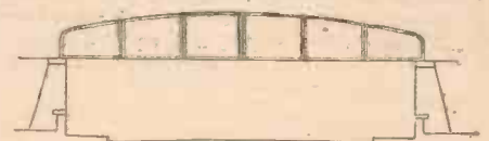
Fig. 2.—Solid, or plate, girder bridge.
