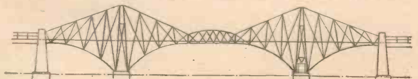
Fig. 3.—Example of cantilever-cum-girder bridge construction.
