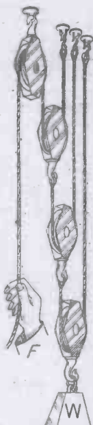
Fig. 17.—First system of pulleys.
