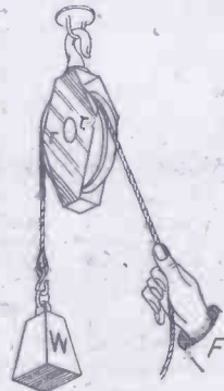
Fig. 11.—Single fixed pulley.
