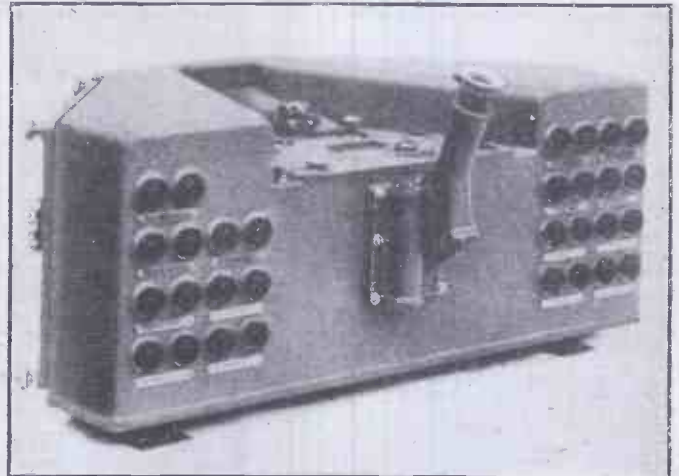
The Avimo Fifteen Channel Camera which records 15 oscillograph traces side by side.
