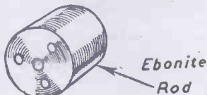
Fig. 4.—(Above) Piece of ebonite rod for making the commutator.
