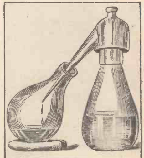
An alchemical distillation apparatus of Moorish origin. (Sometimes known as a "Moor's Head.")
