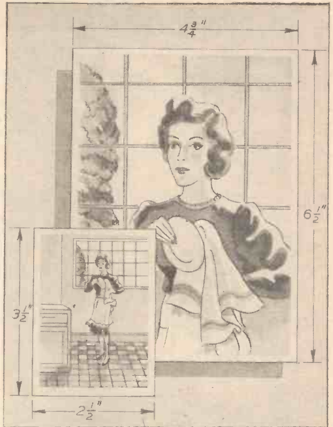
Fig. 12.—Showing how a half-plate enlargement can be made from an ordinary "snap" negative.
