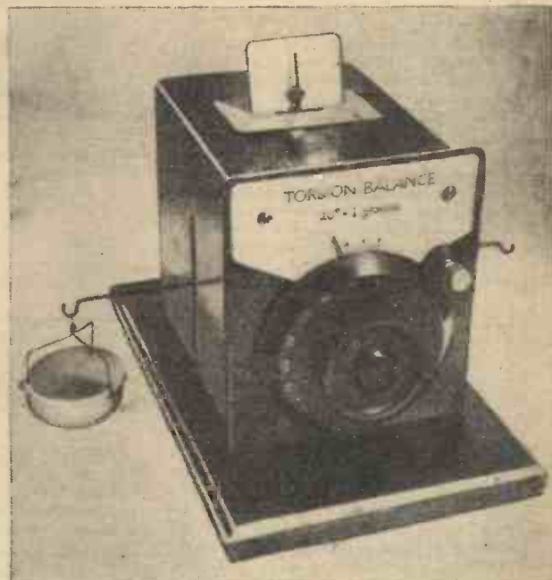
Front view of the completed balance.
