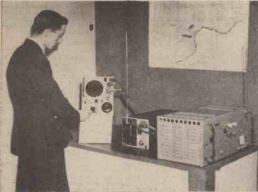
An officer demonstrating the "G" Box. This was used as a navigational aid in aircraft to enable them to pin-point themselves over any predetermined spot.
