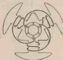
Fig. 4.—Winding diagram for the armature.
