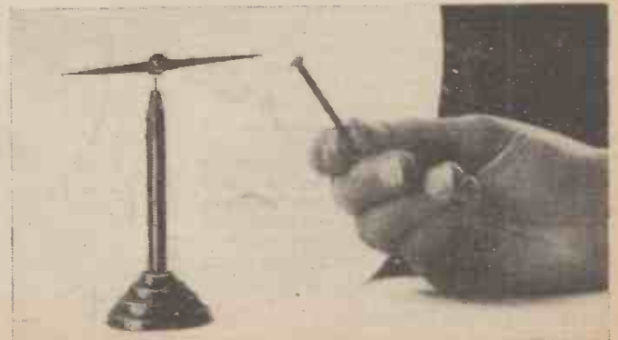
Residual magnetic influence in a nail which has been electro-magnetised, is sufficient to exert its effect upon a compass needle.
