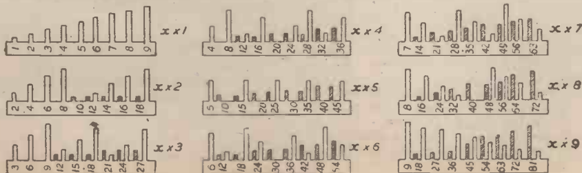
Fig. 21.—The Bollée tongued plate system.
