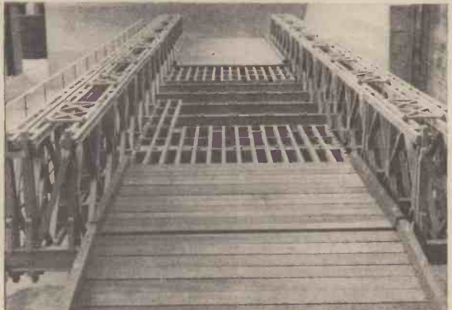
A section of a Bailey Bridge model, partly erected in the Bassett-Lowke works at Northampton.
