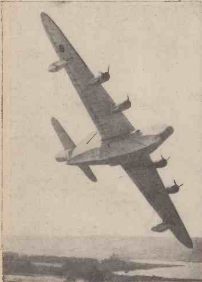
A fine underside view of the Shetland flying-boat undergoing its trials. This new 58-ton air cruiser, largest British 'plane, has been built by Short Bros. and Saunders-Roe. It can carry up to 70 passengers, has a top speed of 267 m.p.h., and four engines of 2,500 h.p. each. Wing span is 150ft., length 110ft.
