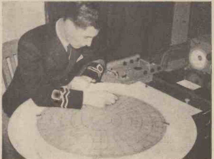
The "Skiatron," used in the Navy for tactical plotting by radar. The instrument is attached to long range warning set, and used in aircraft carriers by the fighter direction officer to control fighters.
