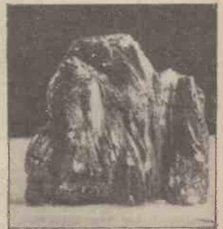
Amber, or "electron"—the natural fossil resin from whose name the word electricity is derived. When rubbed it acquires the power of electrical attraction.
