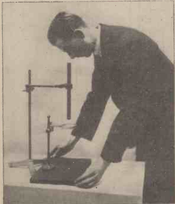
Fig. 12. - View illustrating optical principle of torsionmeter.
