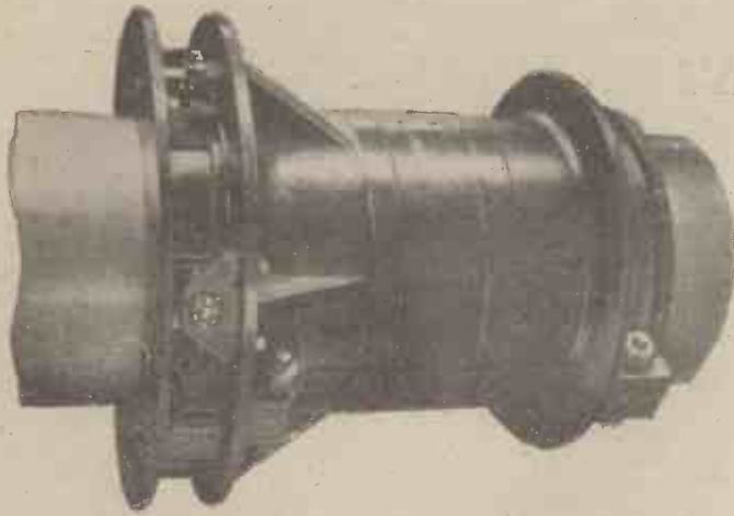
Fig. 3.—Torsionmeter mounted complete on a shaft.
