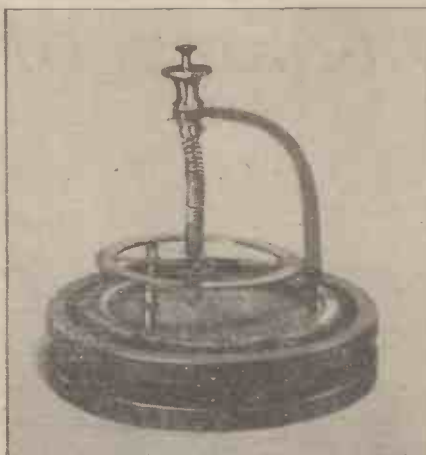
A non-mercurial thermometer used by Dalton. Made about 1800, it comprised one of the world's first metallic-strip thermometers.
