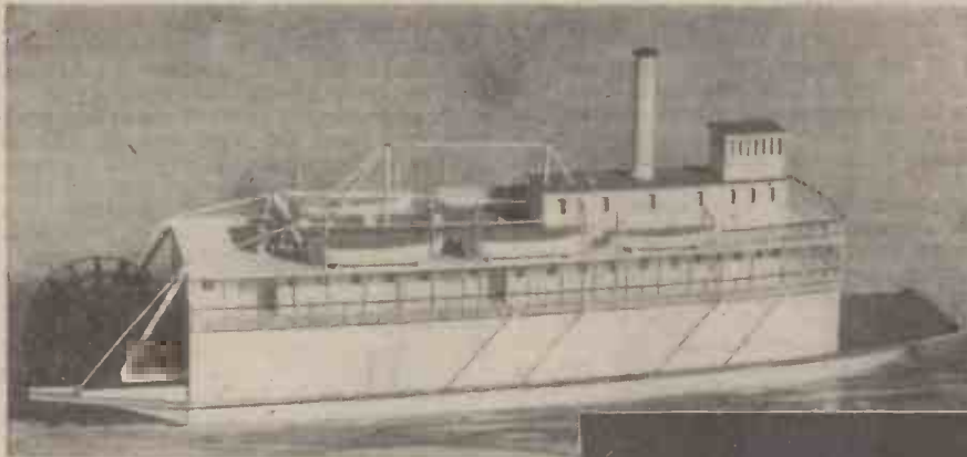
Fig. 4.—Great Lakes steamer, with stern wheel drive, scale 25ft. to 1in.
